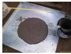
High slump SCC concrete ensures total fill and zero voids
